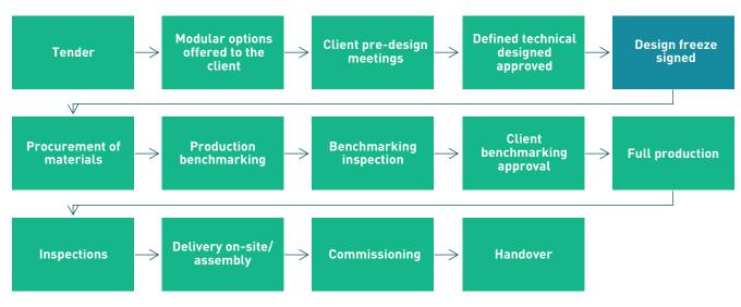
Figure 3.6: Current MMC Manufacturing Supplier Tender to Delivery Process
