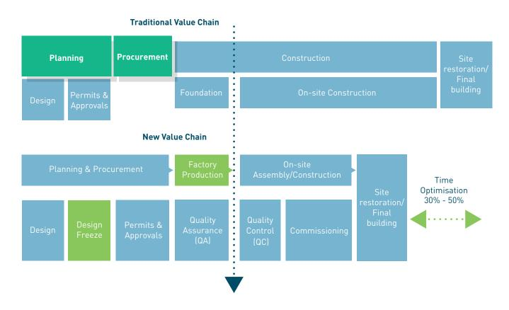
Figure 3.5: MMC Construction Value Chain – Re-imagined (the future state)
